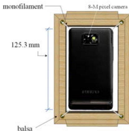
Figure 4. Vibration-proof device designed to reduce high-frequency vibrations in an electric glider. The smartphone is attached to the balsa framework with monofilament.
