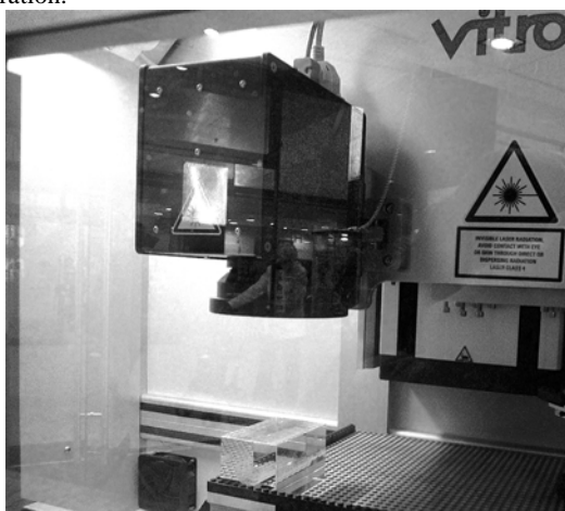
Figure 11. VITRO crystal laser engraving machine of company LOOXIS (Hannover, Germany); courtesy R.Titze (photography by W.Schuhr) (similar: CERION)
