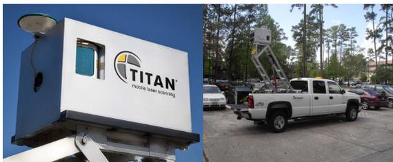
Figure 1. TITAN mobile laser scanning system.
