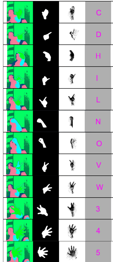
Fig. 9. Snapshots from real-time application showing the original range image, the segmented hand blob and the recognized hand postures
