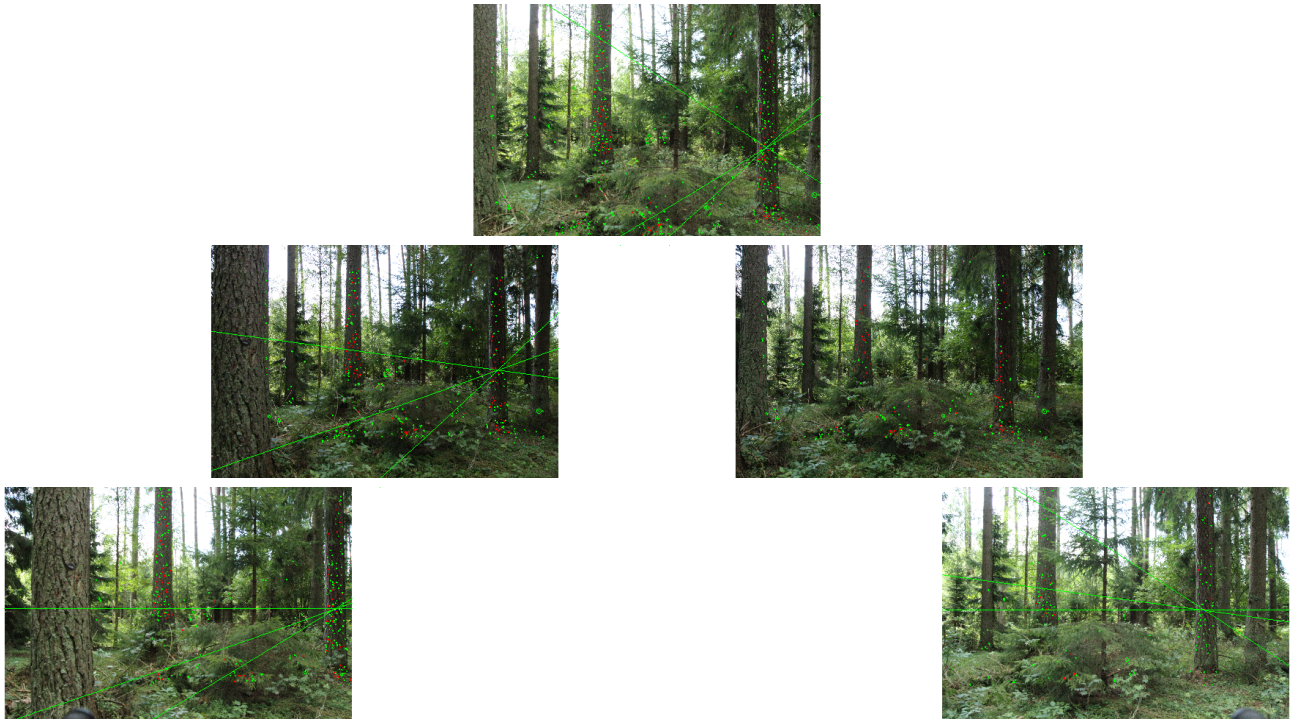
Figure 4: A set of images from the five-camera rig. The relative positioning of the images indicate the relative position of the camera within the rig. The green lines are the epipolar lines for one point.
