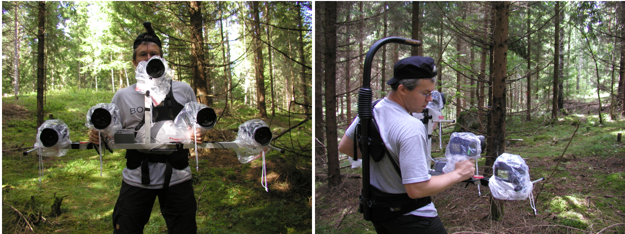
Figure 1: The five-camera rig in the field, carried with Easyrig 2.5.
