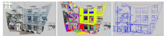
Figure 3. Left: Point Cloud data, Middle: Segmentation result, Right: 3D Edge detection result
