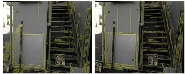
Figure 5. Edge Detection Result Left : Canny Detector, Right: Our System
