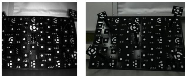
Figure 5. Calibration image for PMD camera (left) and RGB camera (right)
