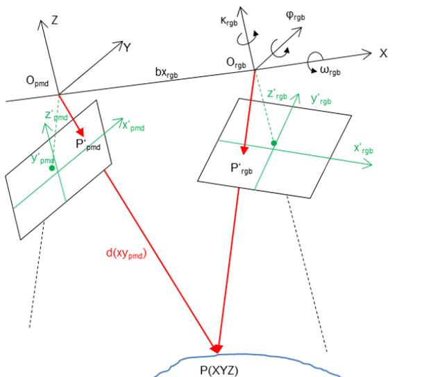
Figure 2. Camera and object coordinate system
