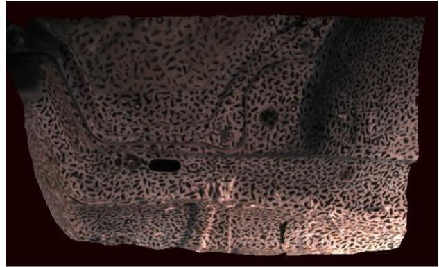
Figure 9. Orthophoto of footwell scene with ground sample distance of 1 mm
