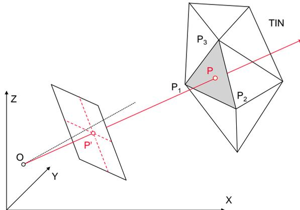
Figure 4. Principle of 3D monoplotting
