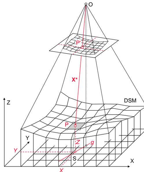
Figure 3. Principle of 2½ D monoplotting
