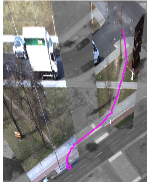
Figure 6: Example of a tracking in the reference coordinate system. Both camera images are transformed onto the ground plane. The ground plane is indicated with an aerial image of the area.
