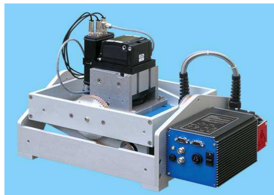
Figure 5: mid-format camera on the gyro stabilised platform AeroStab-2
