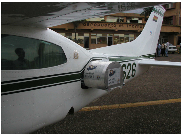
Figure 10: external mounted camera box in Bolivia, used for monitoring Coca plants
