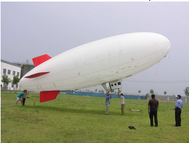
Figure 2: He-Blimp of the University Beijing with a stabilised platform as a carrier for a mid format aerial metric camera (Rollei AIC).
