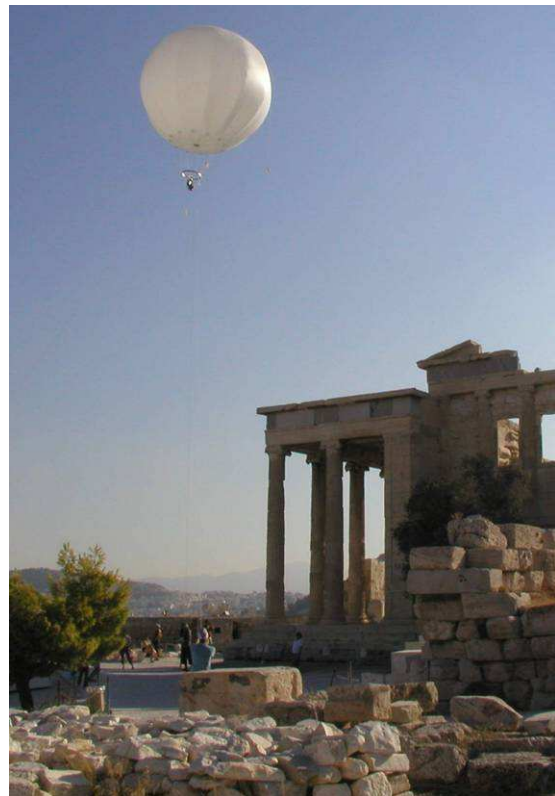
Figure 1: Balloon-photogrammetry for the Acropolis Athens in Greece
