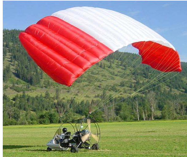
Figure 3: a paratrike with an exciter as a carrier system for airborne Lidar
