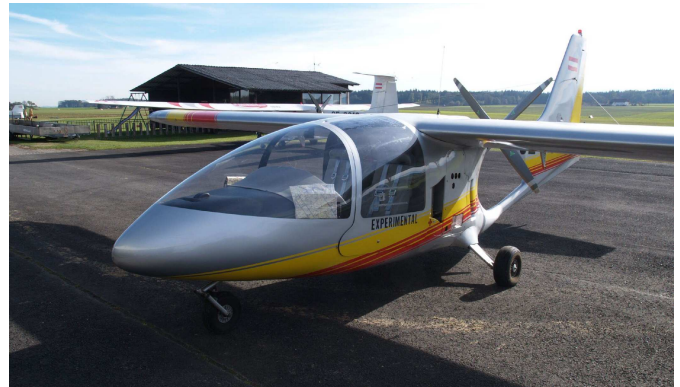
Figure 8: Experimental aircraft of the company Pauly Luftbild-fotographie. Camera and stabilizer was mounted outside in a carbon box
