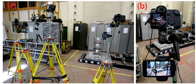
Figure 3: (a) Experimental configuration. (b) A close-up photograph of an individual image station; the mobile phones were mounted on customized tripod mounts.
