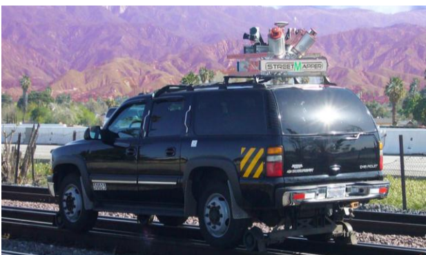
Figure 3: StreetMapper operated on a hi-rail gear vehicle (Photo: Terrametrix LLC, Omaha, NE, USA)
