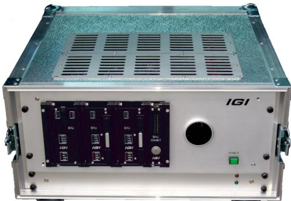
Figure 7: RailMapper control rack
