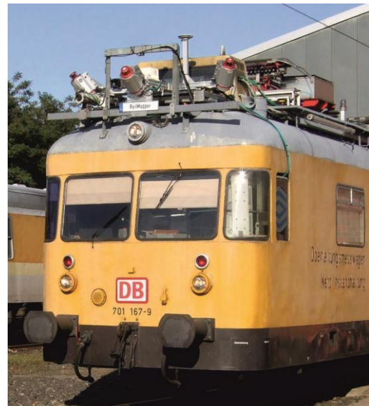
Figure 8: RailMapper sensor assembly with three laser scanners operated on a "Diagnose VT" of the Deutsche Bahn AG
