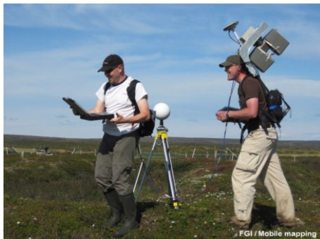
Figure 6. Mapping of permafrost palsa landforms in Finnish Lapland with Akhka backpack mobile laser scanning unit.
