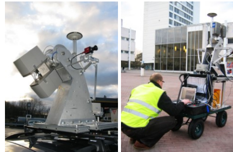
Figure 1. Left: ROAMER as a vehicle MLS (Photo courtesy Hannu Hyypä). Right: Trolley MLS installation.
