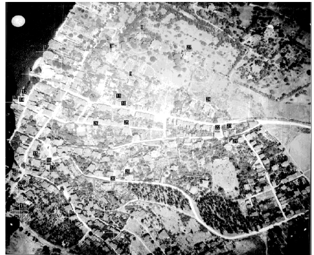
Figure 2. The distribution of the control points in the aerial photo
