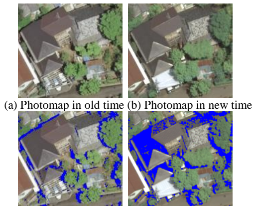
(a) Photomap in old time (b) Photomap in new time (c) Shaded region in old time (d) Shaded region in new time Fig.4. Result part of shaded region extraction in Site1
