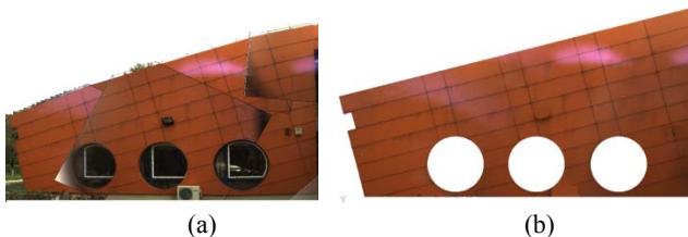
Figure 11. A plan that is part of the front façade of the building (a) The digital image (b) The surface textured by using the presented algorithm
