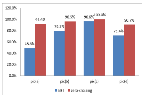
Figure 3(c) matching correct rate of SIFT algorithm and zero-crossing algorithm. Blue bar for SIFT algorithm and red bar for zero-crossing algorithm. The x-axis showed different group of test images and the y-axis stands for the matching correct rate.
