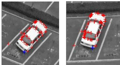
Figure 5 (b) matching result by improved algorithm, red cross for corresponding point, blue crosses for one pair of corresponding points
