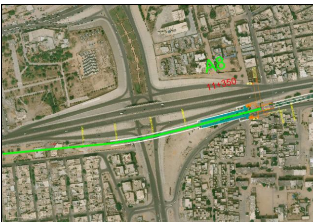
Figure 9. Metro line aligned avoiding a traffic node
