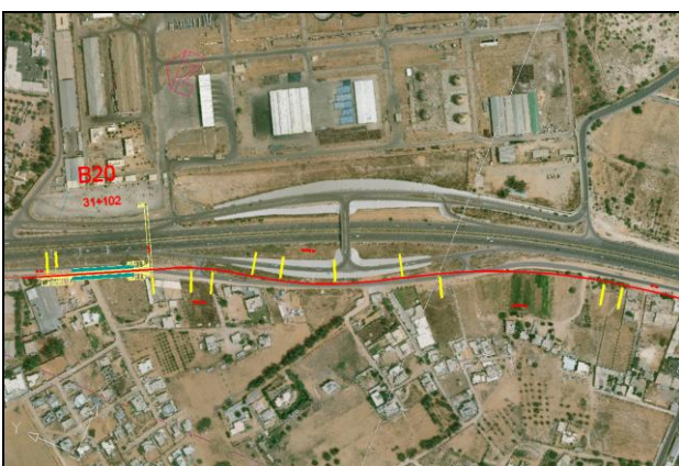
Figure 10. Metro line aligned avoiding bridge foundations
