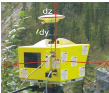
Figure 4. GPS receiver with the ILRIS GPS mount kit set placed on the scanner. Scanner reference system and offsets ( $dy$ ,  $dz$ ) between antenna phase center and scanner origin are represented.
