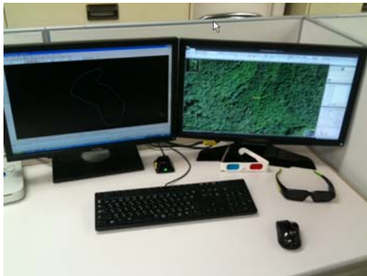
Figure 1. Hardware configuration using the NVIDIA 3D Vision (using dual LCD)
