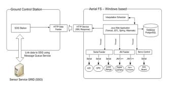
Figure 2. System Diagram and Architecture
