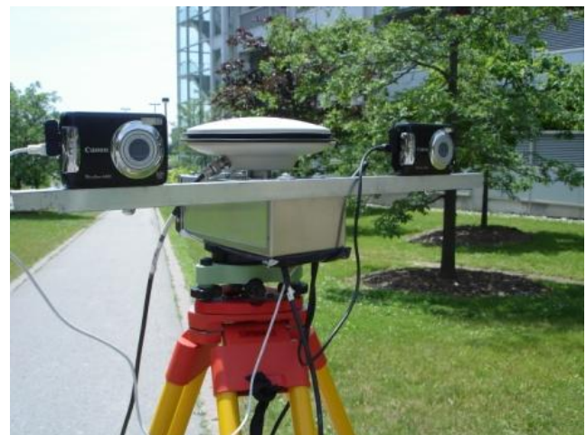
Figure 1. Mobile stereo-mapper system
