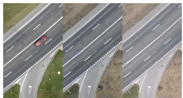
Figure 9: Aspect of orthoimage. Left: reference, Middle: SocetSet, Right: Pix4D
