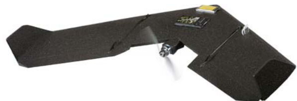
Figure 1: The Swinglet from Sensefly. The wingspan is only 80cm and the total weight including sensing device is 500g.
