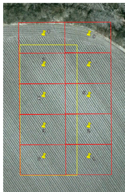
Figure 4: The area (yellow) and the resulting waypoints (yellow pins) with the calculated field of view of the camera (red, overlap is not displayed) in GoogleEarth ®
