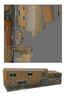
Figure 12. Texture components and the 3D-Model derived from UAV images of the HXE-building at Campus Science City Campus ETH Hoenggerberg, displayed in VRMLVIEW
