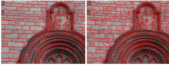
Figure 2. Extracted edges using different Canny's thresholds.
