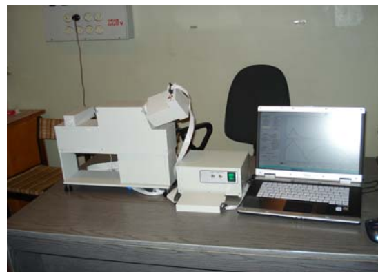
Figure 1. High precision real-time Multi-channel spectrellipsometer.
