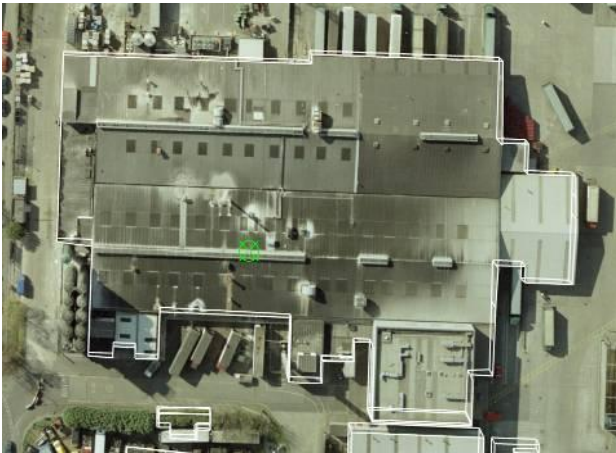
Figure 3. A complex building with more than 50 sides, extracted from a LIDAR point cloud: stereo images are used only to verify the accuracy of the extracted building.
