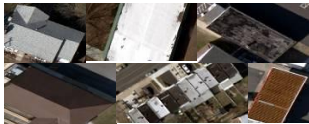
Figure 1. Six different building colors and patterns from one image with a GSD 0.14': a supervised building region growing classification would need six signatures. Two (upper-right and lower-middle) cannot be used because they are inhomogeneous.
