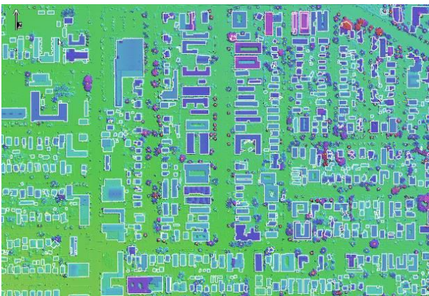
Figure 12. Rectangular buildings and houses easily extracted.
