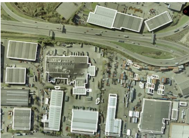
Figure 4. AFE extracted 59 buildings and 13 trees from dense LIDAR. White lines are building boundaries.
