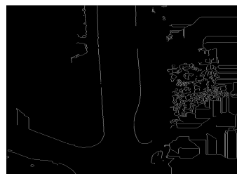
Figure 12. The detected edges using Canny method.
