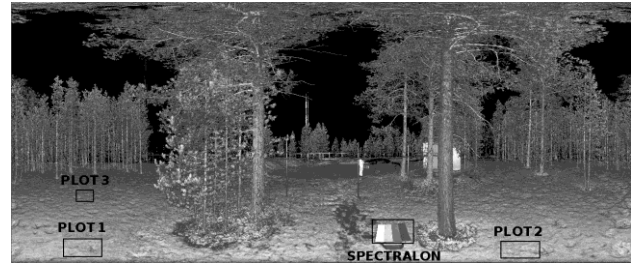
Fig. 1. Intensity image of a measurement from Tähtelä. The square plots 1, 2 and 3 are the sample plots and the Spectralon is the reference panel.
