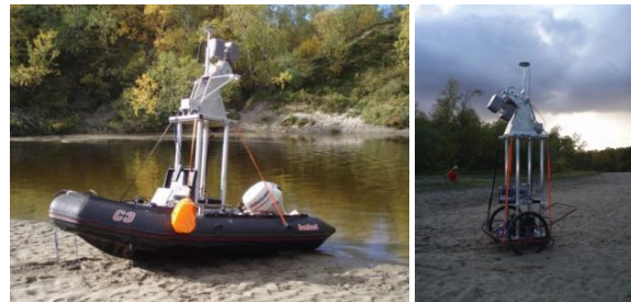
Figure 3. Mobile mapping systems used in this study: a) BoMMS and b) CartMMS
