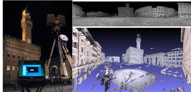
Figure 1. On-the-field Scanning: on Left, the scanner at work; on Top Right, one 360° map; on Bottom Right, one range map imported inside MeshLab.
