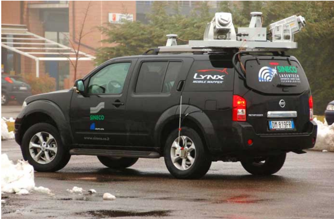
Figure 1 - Van with all the system components
