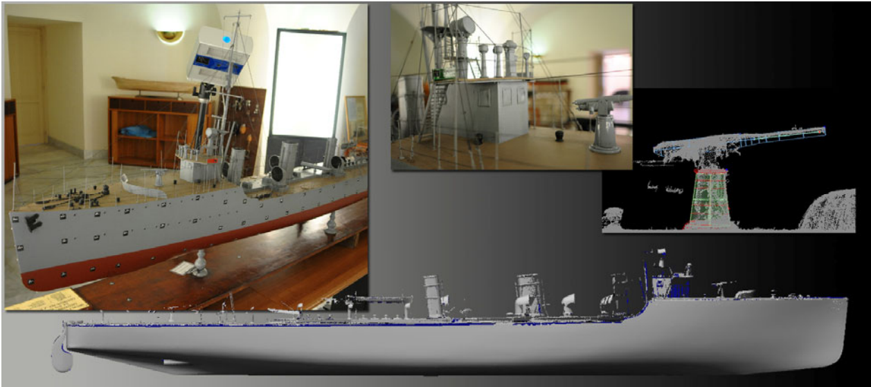
Figure 4: Hybrid survey for 3D modelling of the “Indomito” model of Maritime Museum - Parthenope University of Naples.
