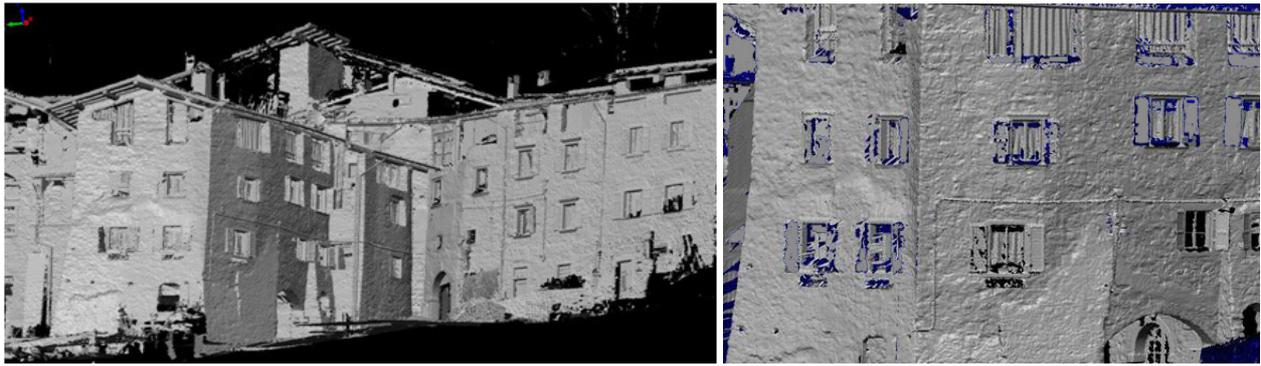
Figure 11: Some 3D results for the Calvola village. For such complex structure, the hole filling procedure is the most time consuming part of the 3D modeling pipeline.
