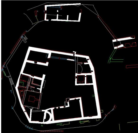
Figure 6: The new map (white and thick walls) of the heritage derived from the range-based 3D model, superimposed onto the old cadastral map.
