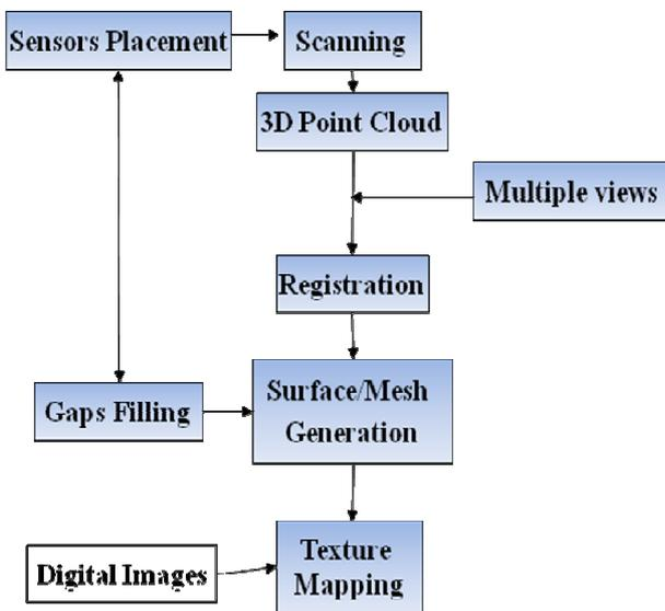
Figure 3: The employed range-based methodology for large and complex structure 3D surveying and modeling
