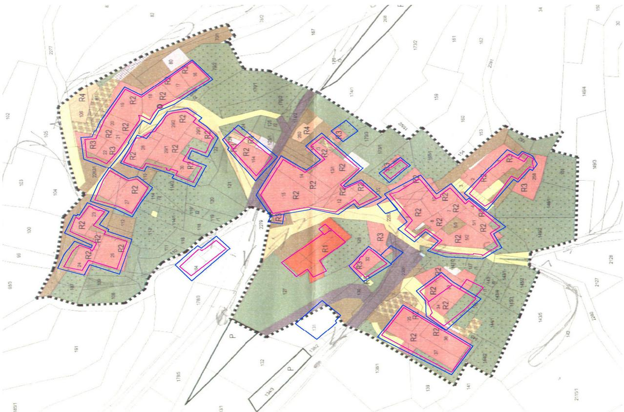
Figure 13: The superimposed building contours (derived from the laser scanning data) onto the existing map of the village. Remarkable shifts and differences are clearly visible.
