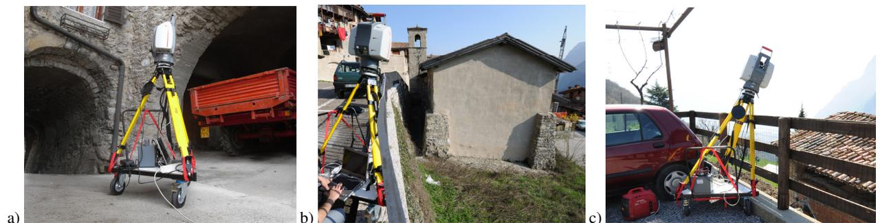
Figure 10: The laser scanner on the home-built trolley (a). Not-accessible areas which required to place the surveying instrument is difficult positions (b, c).
