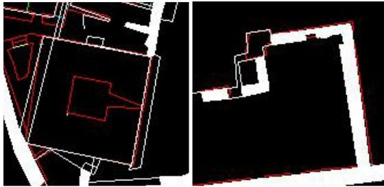
Figure 7: Some differences between the two maps, due to low resolution surveying but also structural changes (in white the more accurate and detailed range-based results).
