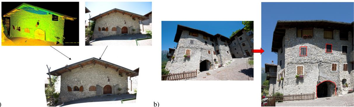
Figure 12: Range and image data co-registered to create an orthophoto of the façade (a). Produced orthophoto and vectorialization of architectural information (b).
