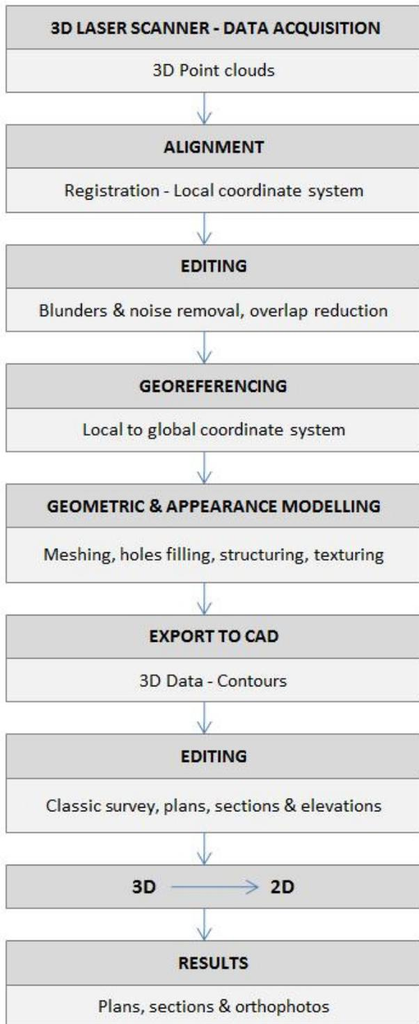
Figure 16: The flowchart of the methodology followed for the 3D surveying of complex heritages and the delivering of 2D results.
