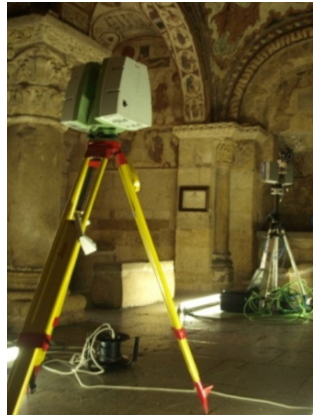
Fig 1. Leica ScanStation C10 and Faro Photon 80 face to face.
