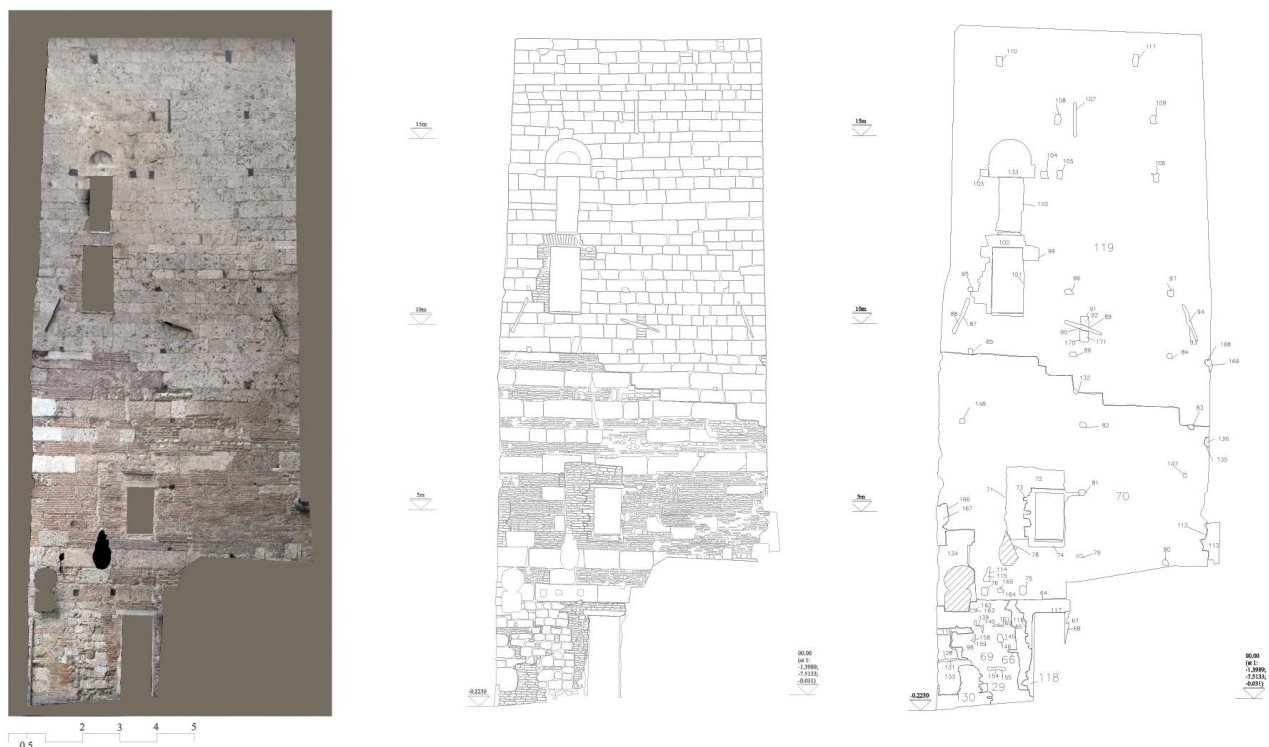
Figure 1. Orthophoto, vectorial drawing of construction materials and “stratigraphic reading.” (elaborated by Rossella Pansini)
