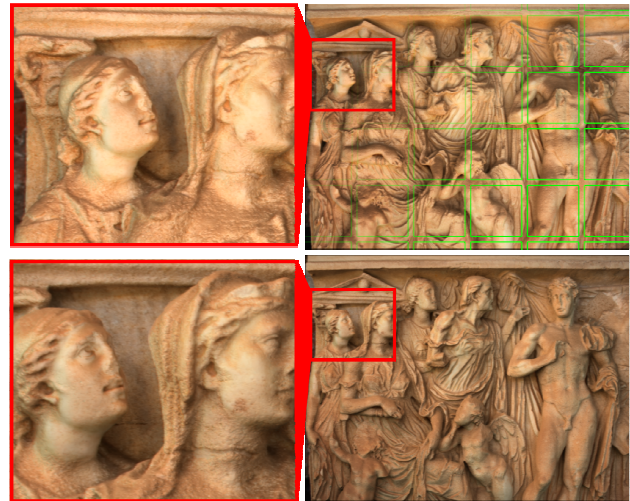
Figure 7. A Polynomial Texture Map is visualized in a multi-resolution fashion. As the user moves the mouse to change the virtual light source direction, the illumination contribution is recalculated and shown in real-time.
