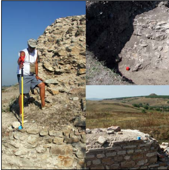
Figure 6. Colored cubes filled with sand had two roles: to help editing the photographic data in PhotoModeler and later to link between the 3D photographic model and the data taken with the total station.
