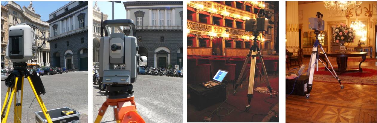
Figure 4 Different instruments employed: GX Trimble, VX Trimble, LS 880 FARO
